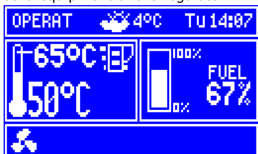
Fig. 18 Auxiliary window with fuel level gauge view.
