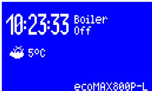
Fig. 5 Regulator screen with boiler off.
